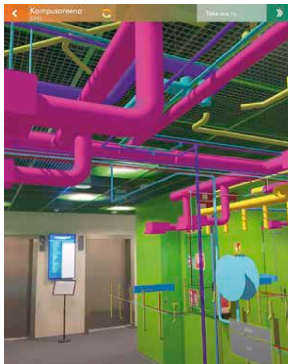
Figure 4: Augmented reality (AR) for facility management to support personnel in the field of operations & maintenance
