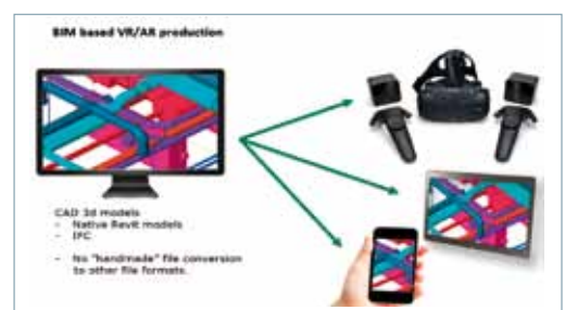
Figure 2. VR/AR models are created from a single source
