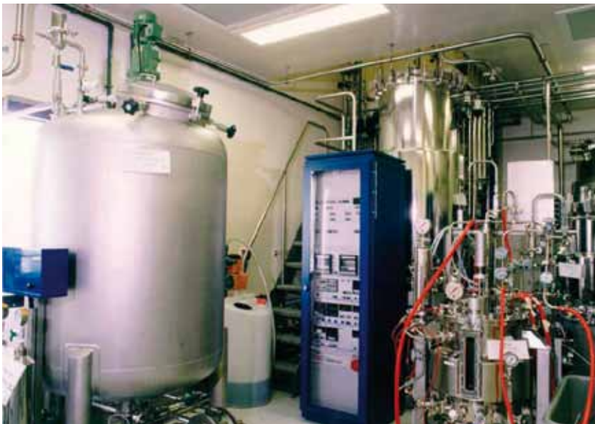
Figure 3: Un-cleanable bioreactor by congestion and poor design
