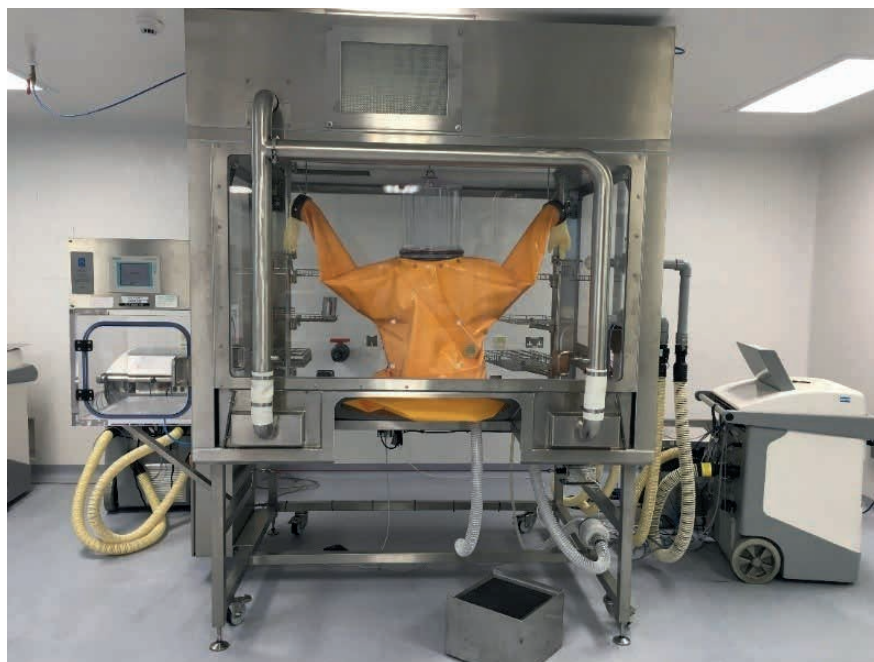
Figure 1 – Sterility testing isolator with “half-suit” and vH_2O_2 gas generator attached
