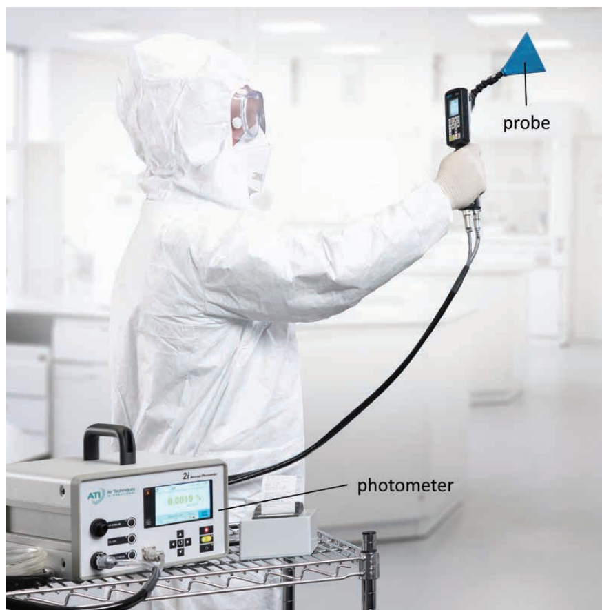
Figure 8.7: Photometer being used with probe and printer
