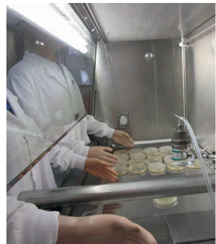
Figure 4: Center Cross Contamination test (left) set up in the presence of three users
