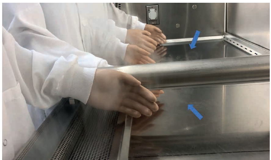
Figure 3: Smoke penetrating the work area in the presence of three users' hands indicating a loss of Product Protection
