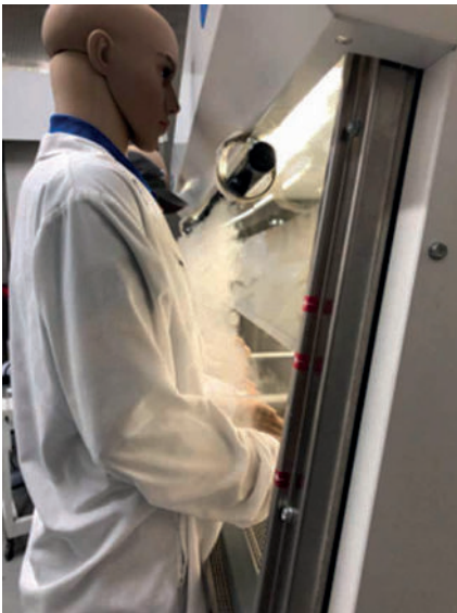
Figure 2a: Construction of a smoke curtain at the front access opening with the mannequins present
