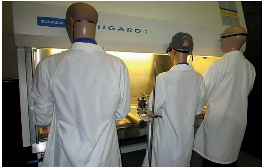
Figure 2b: Placement modification of the NSF International Standard 49 Aerosol Microbiological testing set up in the presence of three users
