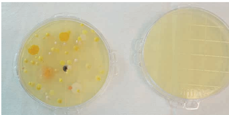
Figure 1: Active air sampling plates pre (left) and post (right) HPV biodecontamination after incubation.
