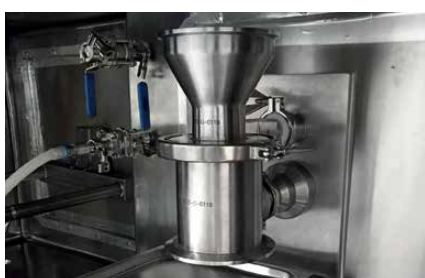
Figure 2: Isolator milling – the milling head is contained within the isolator, with the motor and controls mounted externally (photo Hanningfield Process Systems)
