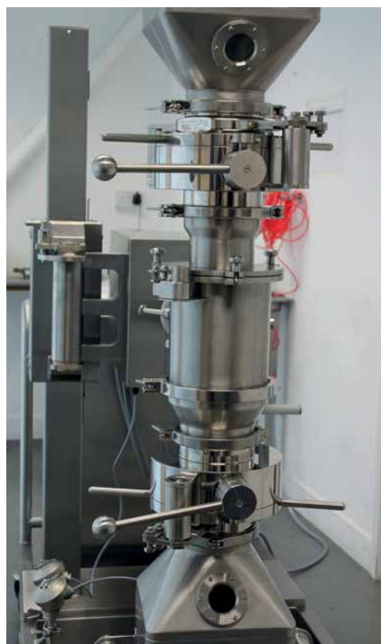
Figure 1: Conical mill with high containment split valves installed on inlet / outlet (photo Hanningfield Process Systems)
